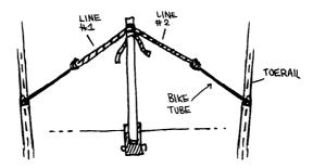
One of the reasons we converted Pino from wheel to tiller was to simplify self-steering. We are big fans of shock-cord sailing, which consists of using a set of shock cords and blocks to self-steer a boat without the need for a windvane.
